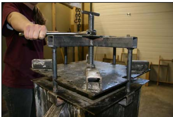
Step 8 – Tightening the nut on the extractor to remove the interior mold
