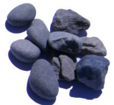
Drainage Gravel 12 mm ( \frac{1}{2} ")
