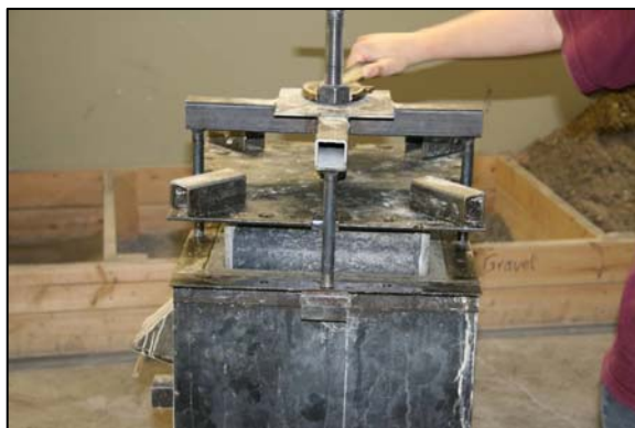
Step 8 – Tightening the nut on the extractor to remove the interior mold
