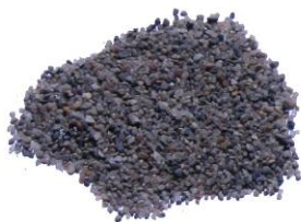
Concrete Sand 1 mm (0.04")
