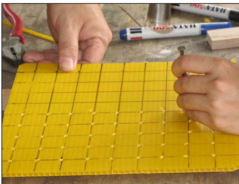
A corrugated plastic diffuser with well placed holes
