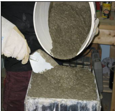
Step 7 - Fill the mold full of concrete
