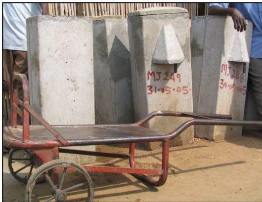
Transporting filters with a specially constructed dolly
